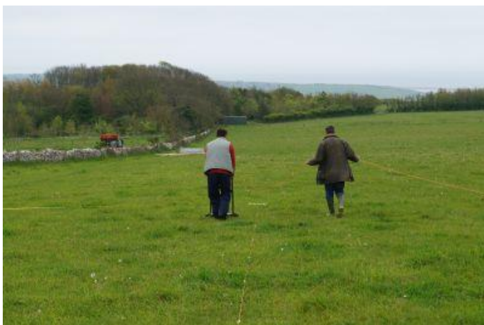
Figure 2: Case study 2: conducting resistivity survey. Image credit: Hayley Roberts
